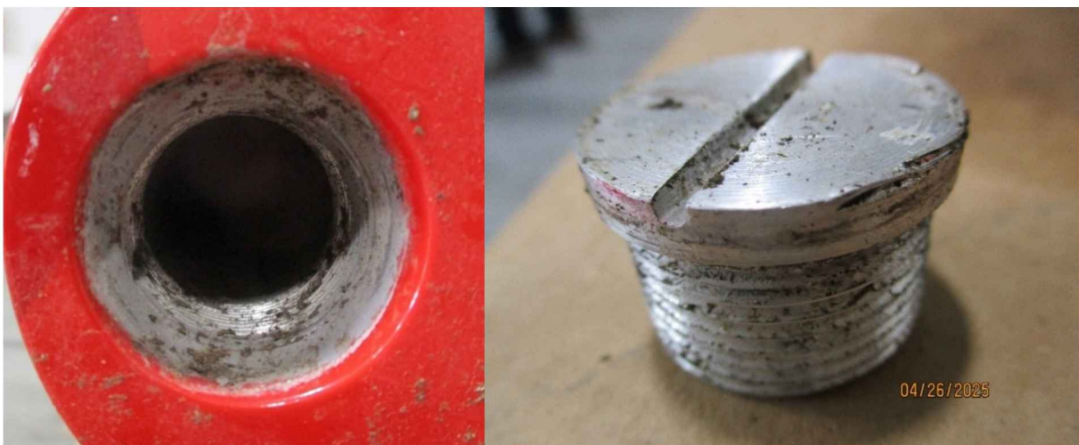
Figure 2. Left elevator counterweight installation hole (left) and recovered counterweight plug (right). Note: gouging and paint transfer on counterweight plug.
